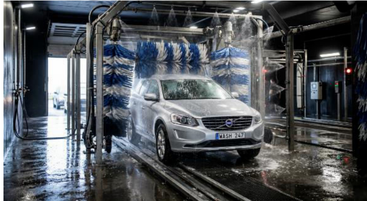
Fig. 3.1: Automated Car Washing System Showing Spraying and Brushing Stages
