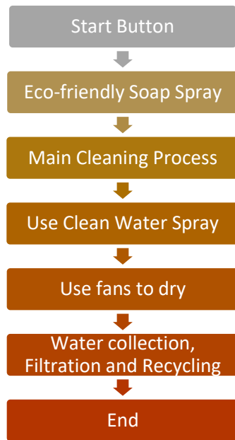
Fig. 4.2: Flowchart of Automatic Car Washing Process
